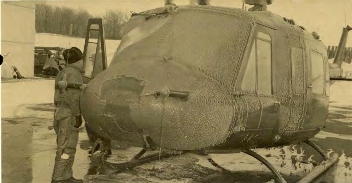
Ice on this helicopter was deposited during test. In flight such a condition as shown could be catastrophic.
